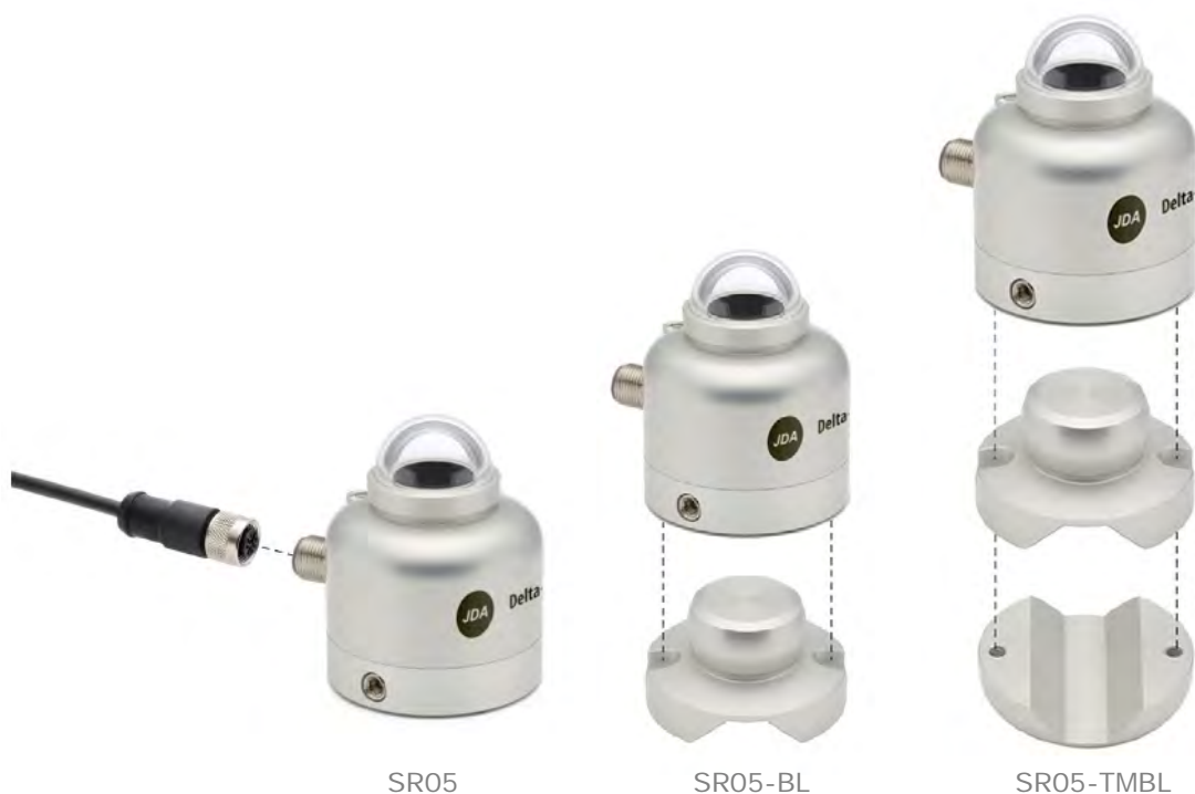
Figure 5.2.1 From left to right: SR05 in its standard configuration with 3 metre cable; with optional ball levelling for easy mounting and levelling on a (non-)horizontal surface; with optional ball levelling and tube mount for easy installation on a 25 to 40 mm diameter tube. Mounting screws are included with the ball levelling and / or tube mount.
