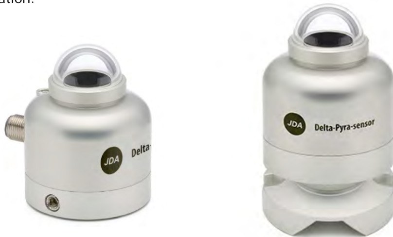
Figure 0.1 On the left SR05-A1 analogue second class pyranometer with bubble level and M12-A cable connector in its standard configuration (3 metre cable standard included); on the right SR05-A1 with optional ball levelling, for easy mounting and levelling on (non-) horizontal surfaces (included mounting screws not displayed)
